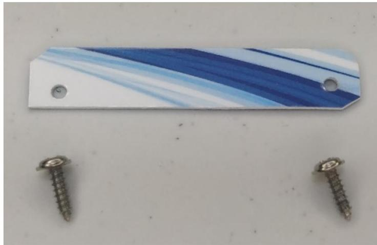
Using an expired credit card or any plastic card cut a link as shown in the image above. The length should be according to the distance between the servo lever and the vent slider. Drill 2 holes such that the screw can freely rotate in the holes. The screws can be found in the servo package.
