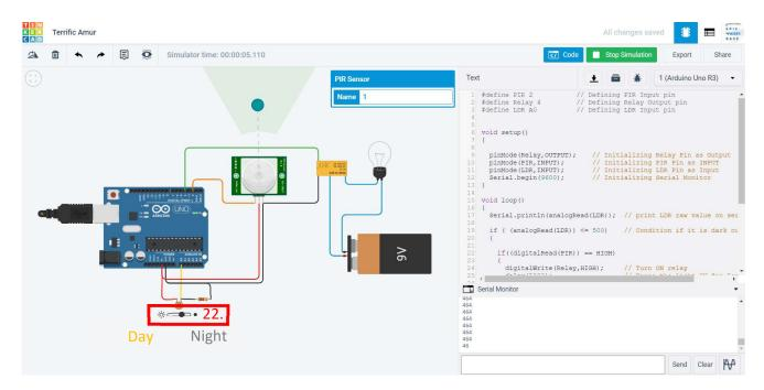
Slide the point on bar towards Day or Night, it detects the brightness intensity. The Raw values can be seen on Serial Monitor. We have identified 500 as threshold in the code. Any value below 500 means it is dark outside and any value above 500 means it is bright.
